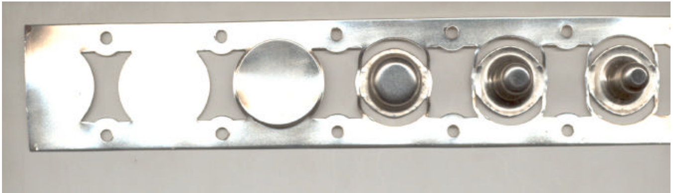
I STAGE II STAGE III STAGE IV STAGE V STAGE VI STAGE Piercing Idle Stage Lancing First Draw Second Draw Third Draw
